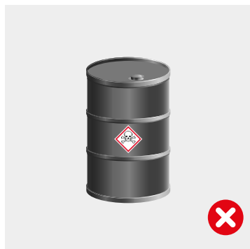
Chemical container without secondary containment
