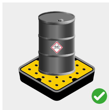
Chemical container with secondary containment
