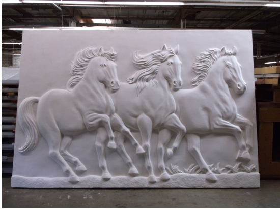
Precast Horses for Soundwall - Southern California
