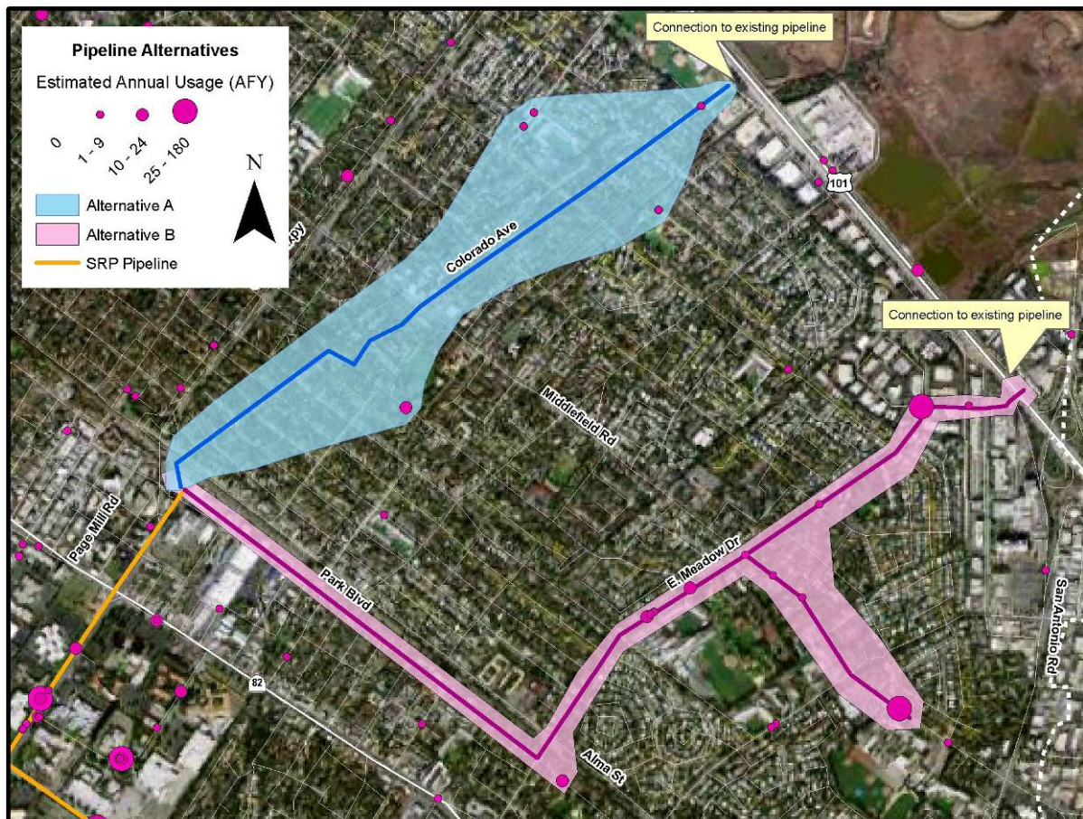
Figure 3-1: Alignment Alternatives A and B
