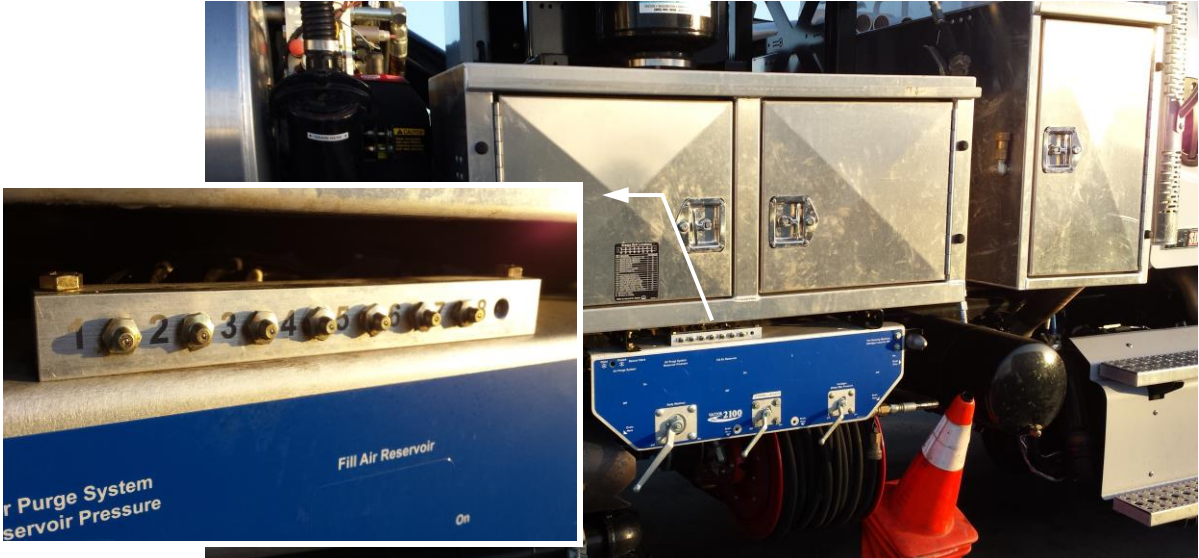
Step 16: Grease Zerks A to H located at the Rear Passenger side
