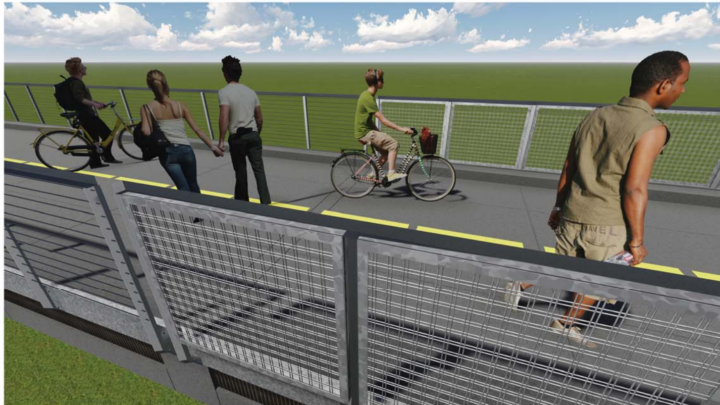
PALO ALTO - HWY 101 PEDESTRIAN / BICYCLE PATH OVERCROSSING (Galvanized cable rail and In-fill Galvanized double wooven wire mesh shown) 3/17/2017
