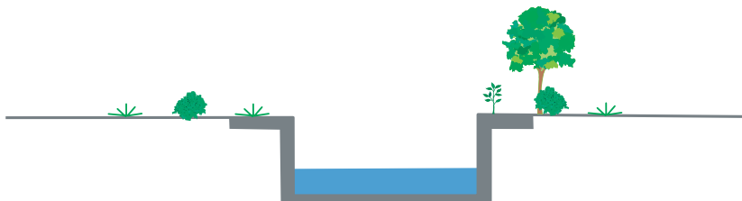
D. Concrete lined channel
