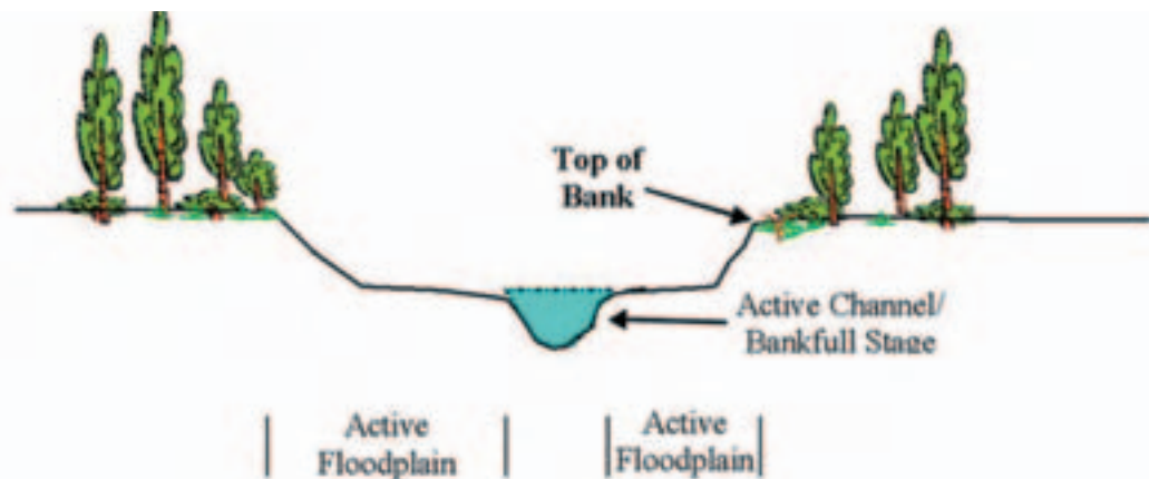
FIGURE 1: CROSS-SECTIONAL VIEW OF A NATURAL STREAM
