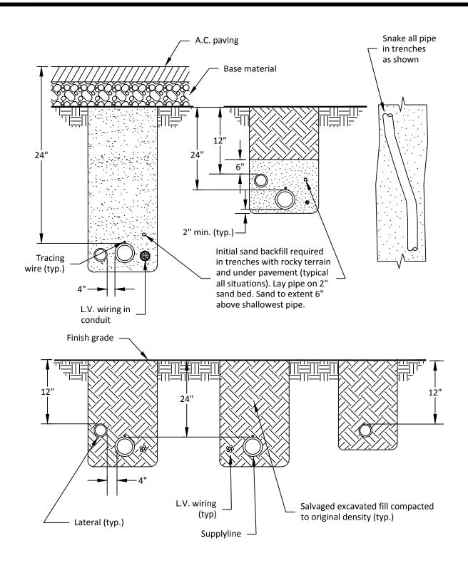
NOTE: Provide 15" cover for rotor system lateral lines. Refer to Tree Technical Manual, Section 2.20.C-D for additional information.
