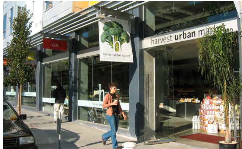
Figure 83 Retail ground floors provides adequate floor to ceiling heights, transparency, and signage.
