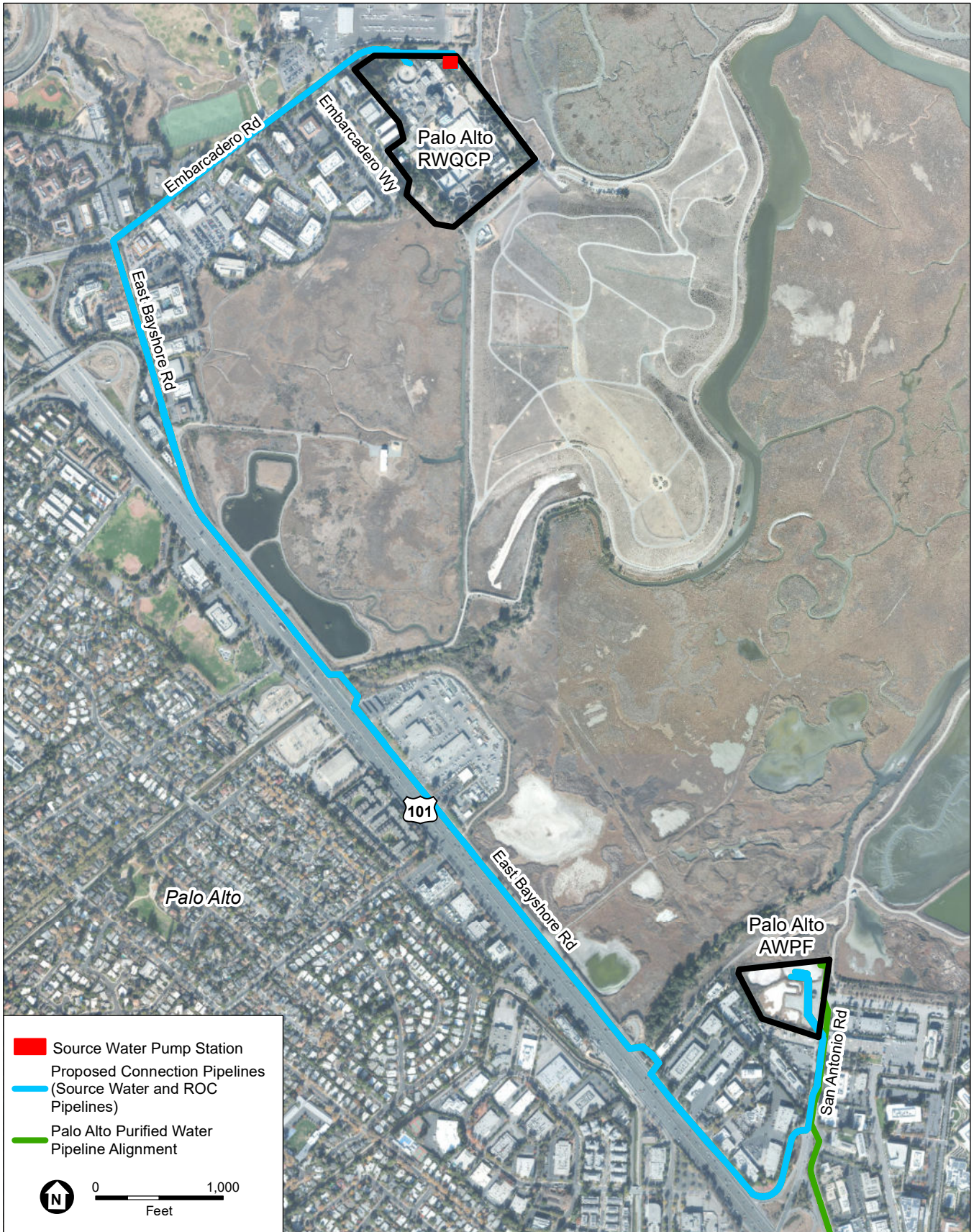
Figure 2-7 Connection Pipelines between the Palo Alto Advanced Water Purification Facility and the Palo Alto Regional Water Quality Control Plant
