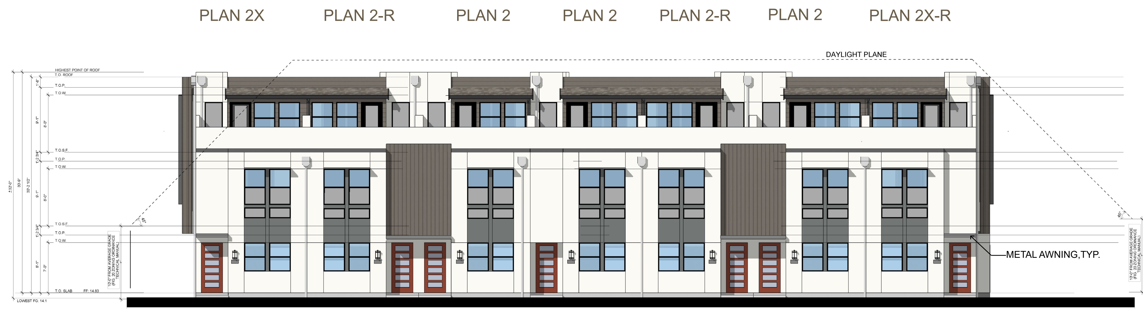
BUILDING 2 - 7 PLEX - FRONT ELEVATION SCALE: 1/8"=1'
