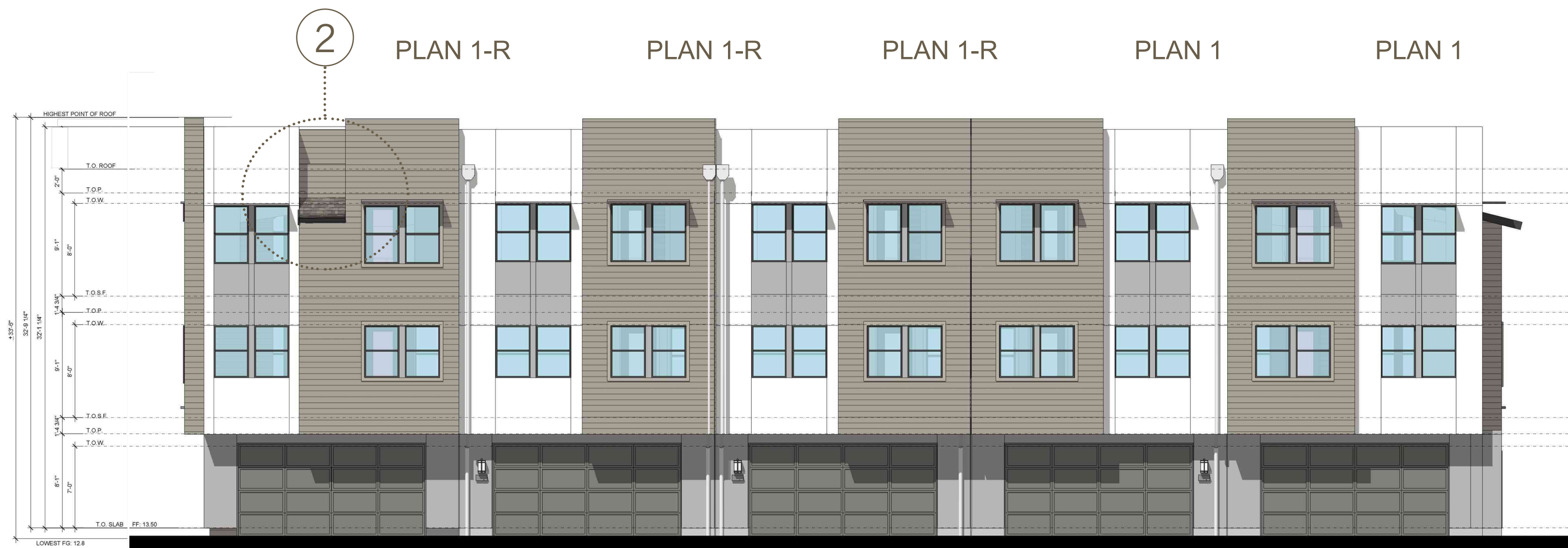
BUILDING 1 - 5 PLEX - REAR ELEVATION SCALE: 1/8"=1'
