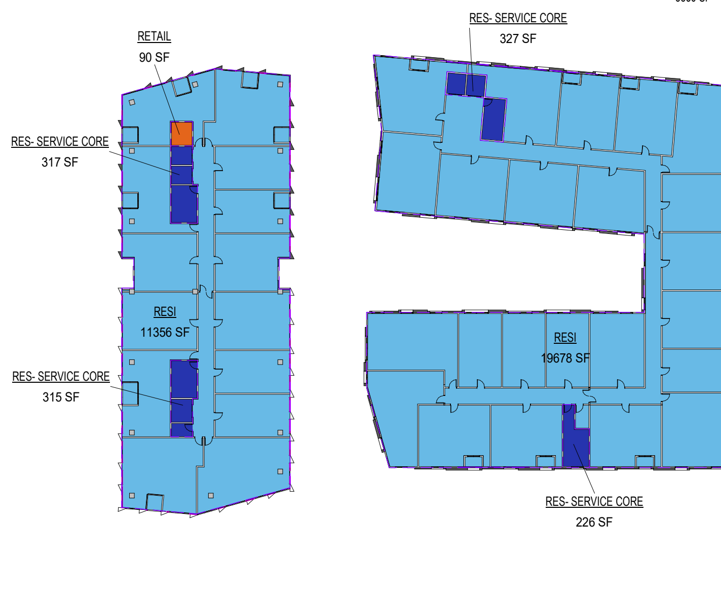
7 ■ Level 5 SEE FLOOR PLAN FOR DETAIL DIMENSION Scale: 1" = 40'-0" (6, & 7TH FLOORS ARE SIMILAR)
