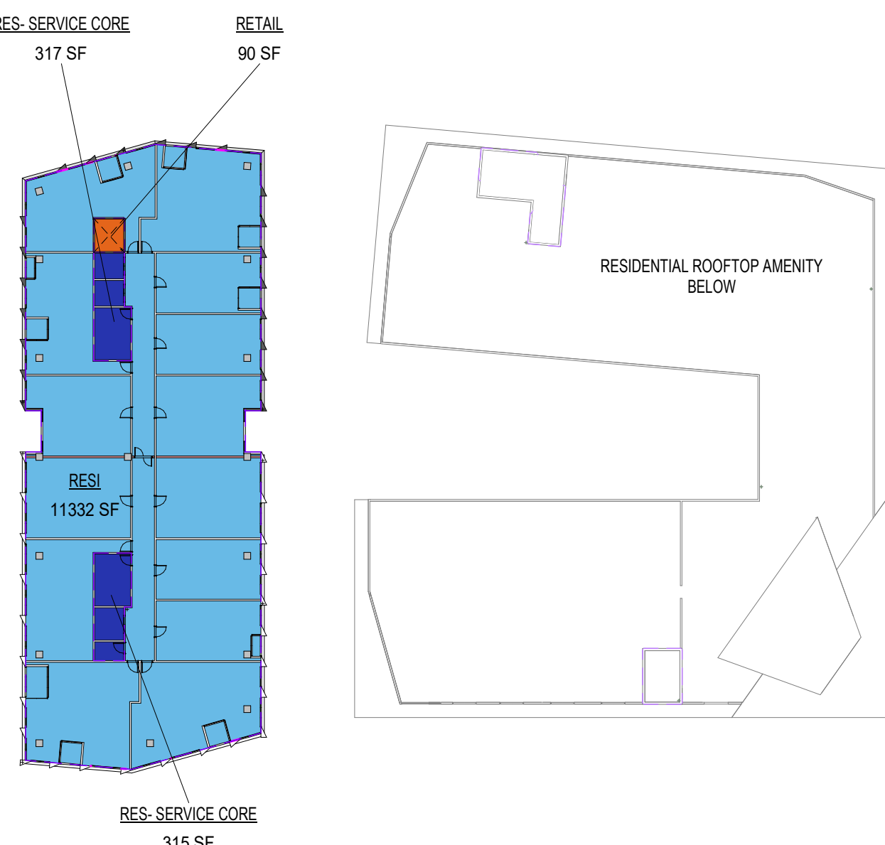
9 ■ Level 9 SEE FLOOR PLAN FOR DETAIL DIMENSION Scale: 1" = 40'-0" (10TH - 16TH FLOORS ARE SIMILAR)
