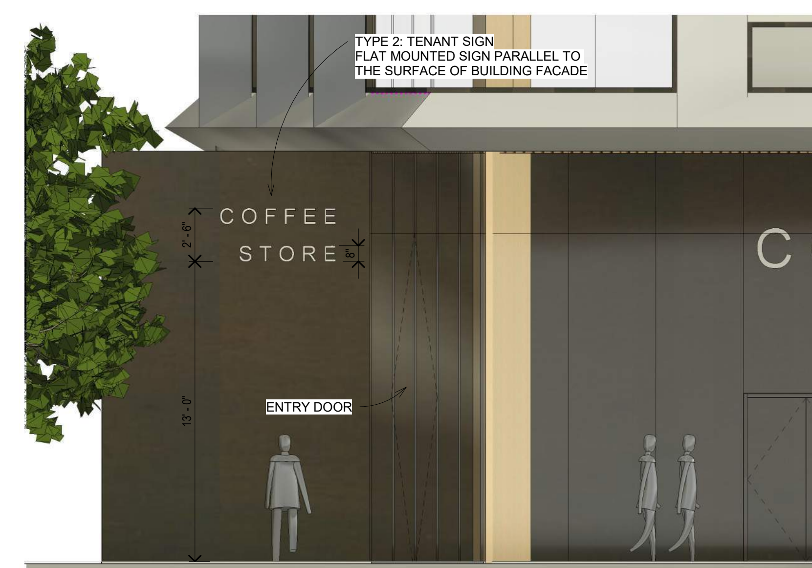
5 SIGNAGE - TOWER A RETAIL Scale: 1/4" = 1'-0"
