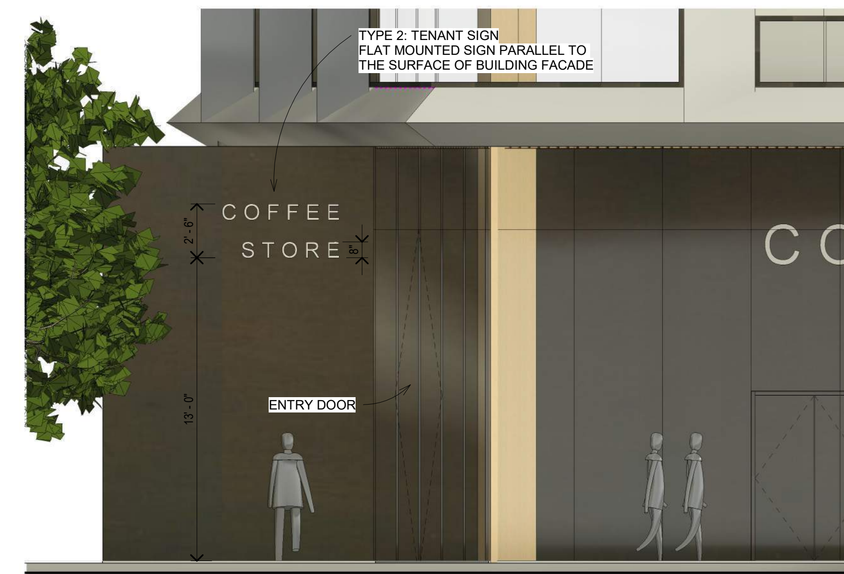
5 SIGNAGE - TOWER A RETAIL Scale: 1/4" = 1'-0"
