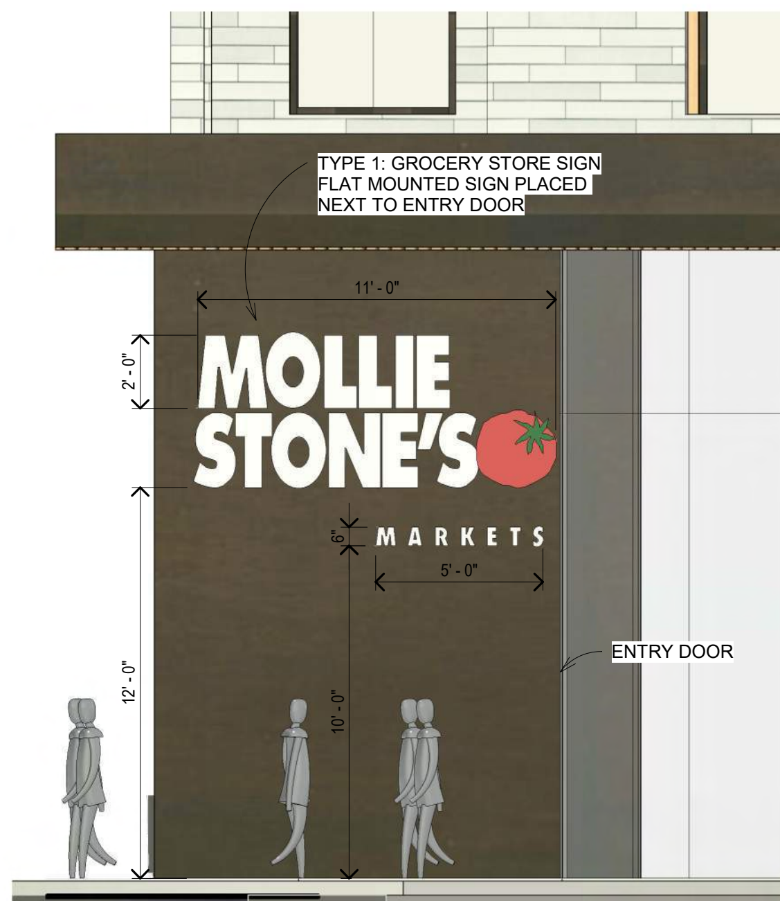
1 SIGNAGE - PODIUM GROCERY STORE ENTRY Scale: 1/4" = 1'-0"
