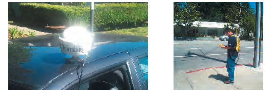
Figure 4.30: Global Positioning Equipment was used for the assessment of travel times.
