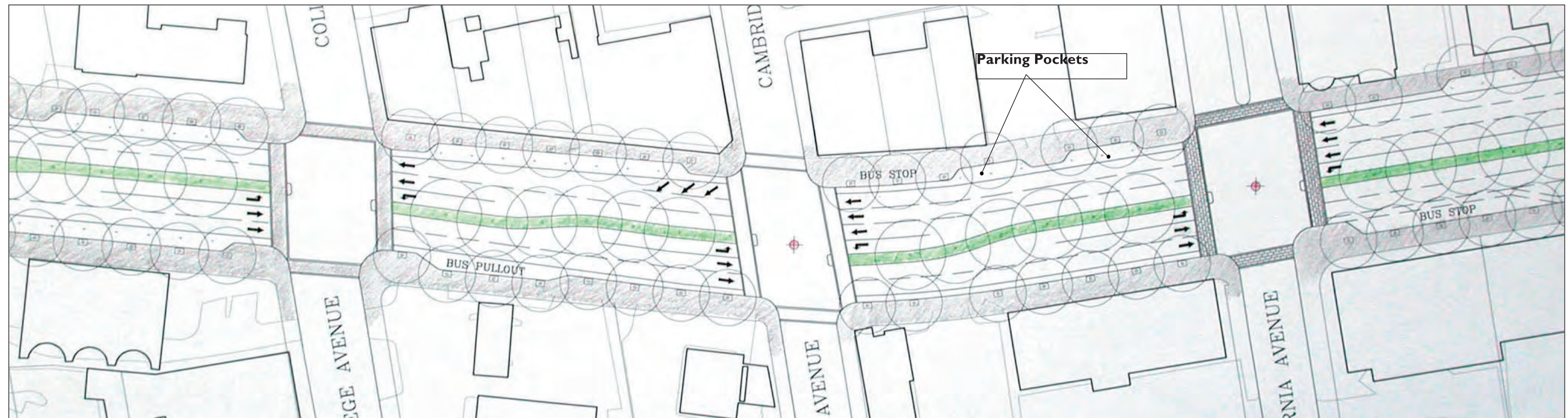
Figure 5.24: Example of a lane reduction from 3 to 2 lanes in northbound direction occurring between Cambridge and College Avenues
