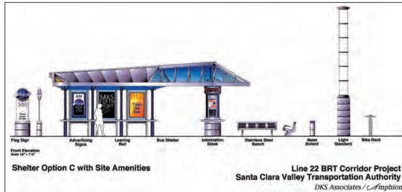
Figure 5.62: A variety of streetscape amenities are proposed for the VTA line 22 BRT Corridor (Conceptual Illustration November, 2001, DKS Associates/Amphion)
