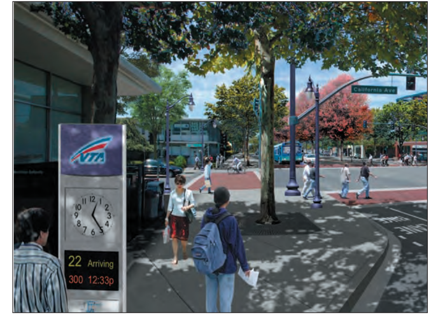
Figure 5.13: The proposed bulb-outs would increase the amount of space available for bus stop improvements and passenger boarding.
