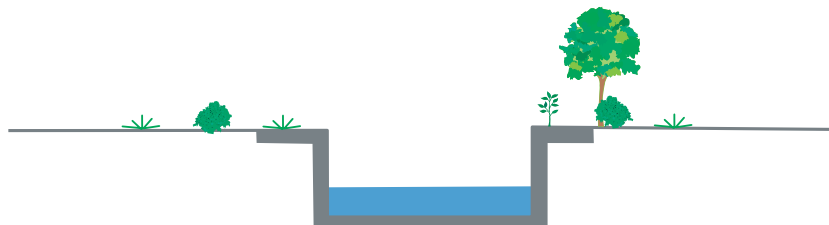
D. Concrete lined channel
