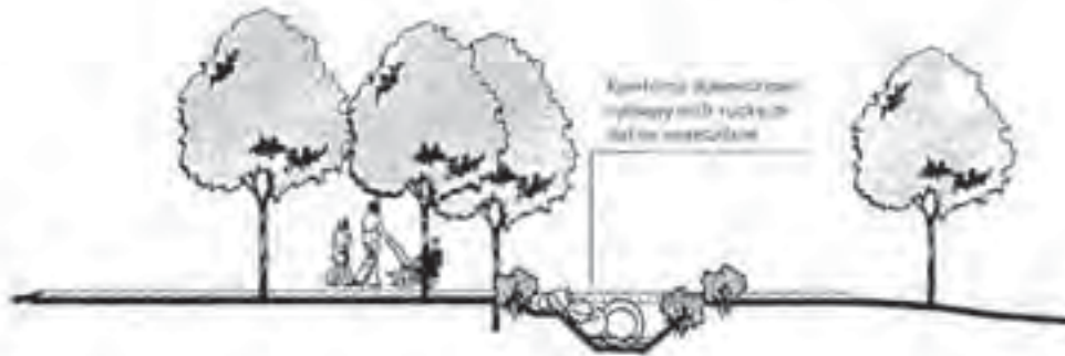
Culvert crossings of small streams and drainages
