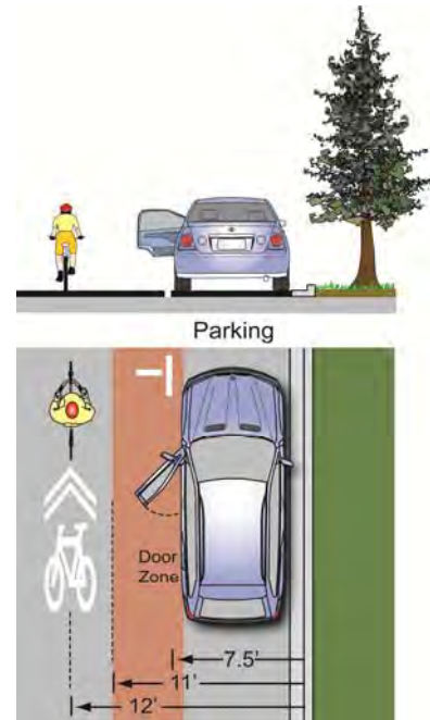
Sharrows delineate bicyclists’ path of travel away from potential open car doors and improve wayfinding.
