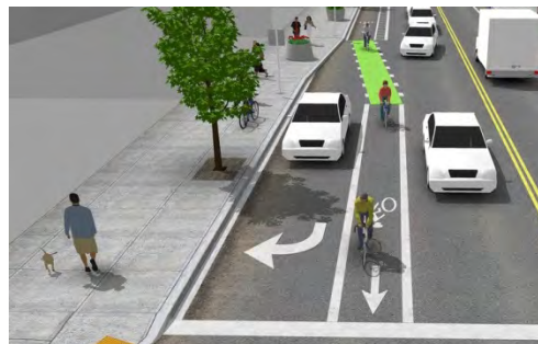
Intersection through markings (far left) and colorized bike lanes (left) are two examples of potential enhancements to existing arterial facilities.
