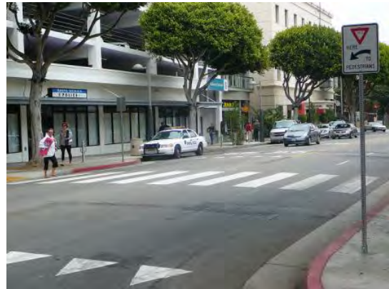
Yield teeth encourage drivers to slow down and watch for pedestrians in a crosswalk.
