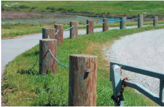
Bollards from re-used utility poles and galvanized chain
