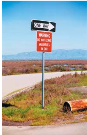
Regulatory signs have a strong visual impact. Their size and color is often subject to traffic engineering standards more appropriate for urban settings. The example is mounted higher than is needed in the flat, treeless Baylands environment.
