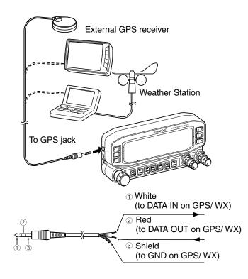
Use an external GPS receiver which conforms to the NMEA-0183 format and is compatible with RS-232C signal polarity output at the below mentioned levels
