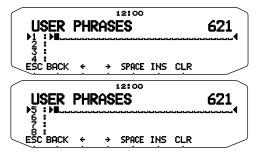
This function (clipboard image) allows you to paste phrases into the APRS message compilation mode. You can create up to 8 phrases each of which can consist of up to 32 characters.
