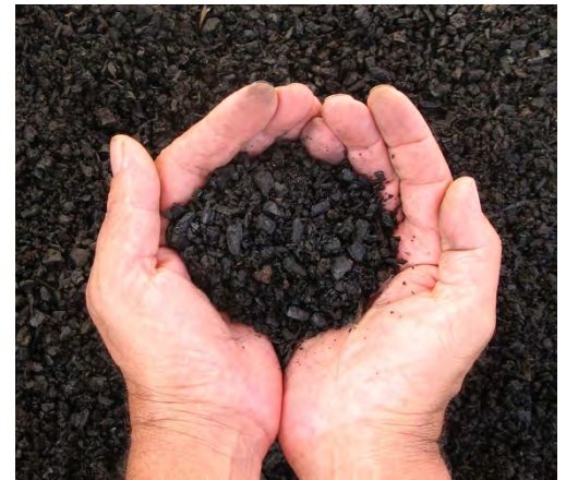
Biochar is charcoal used as a soil amendment. Biochar is a stable solid, rich in carbon, and can endure in soil for thousands of years. Like most charcoal, biochar is made from biomass via pyrolysis. Biochar application to soil is being evaluated as an approach to carbon sequestration.
