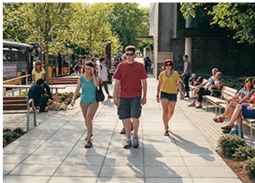
Figure 52 Light colored pavement reduces the urban heat island effect.
