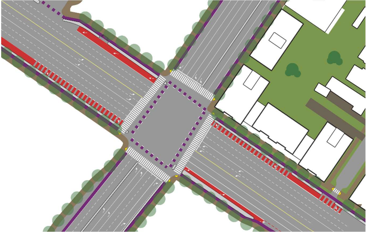
Figure 87 El Camino Real and Page Mill Road Conceptual Intersection Design
