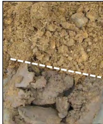
Left: 14" fill soil overlaid compacted clay. Roots were primarily limited to fill soils, which were dry.
