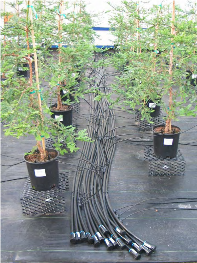
Figure 2. Tree organization, irrigation treatment delivery and expanded metal pot stands.
