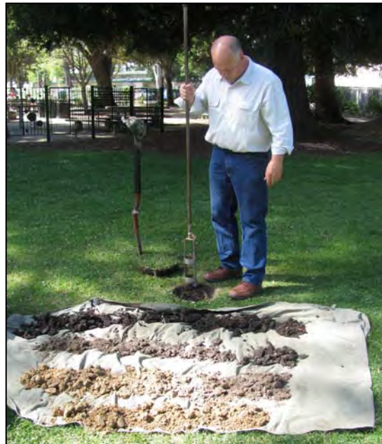
Photo 5: Soils were excavated by hand using a soil auger.
