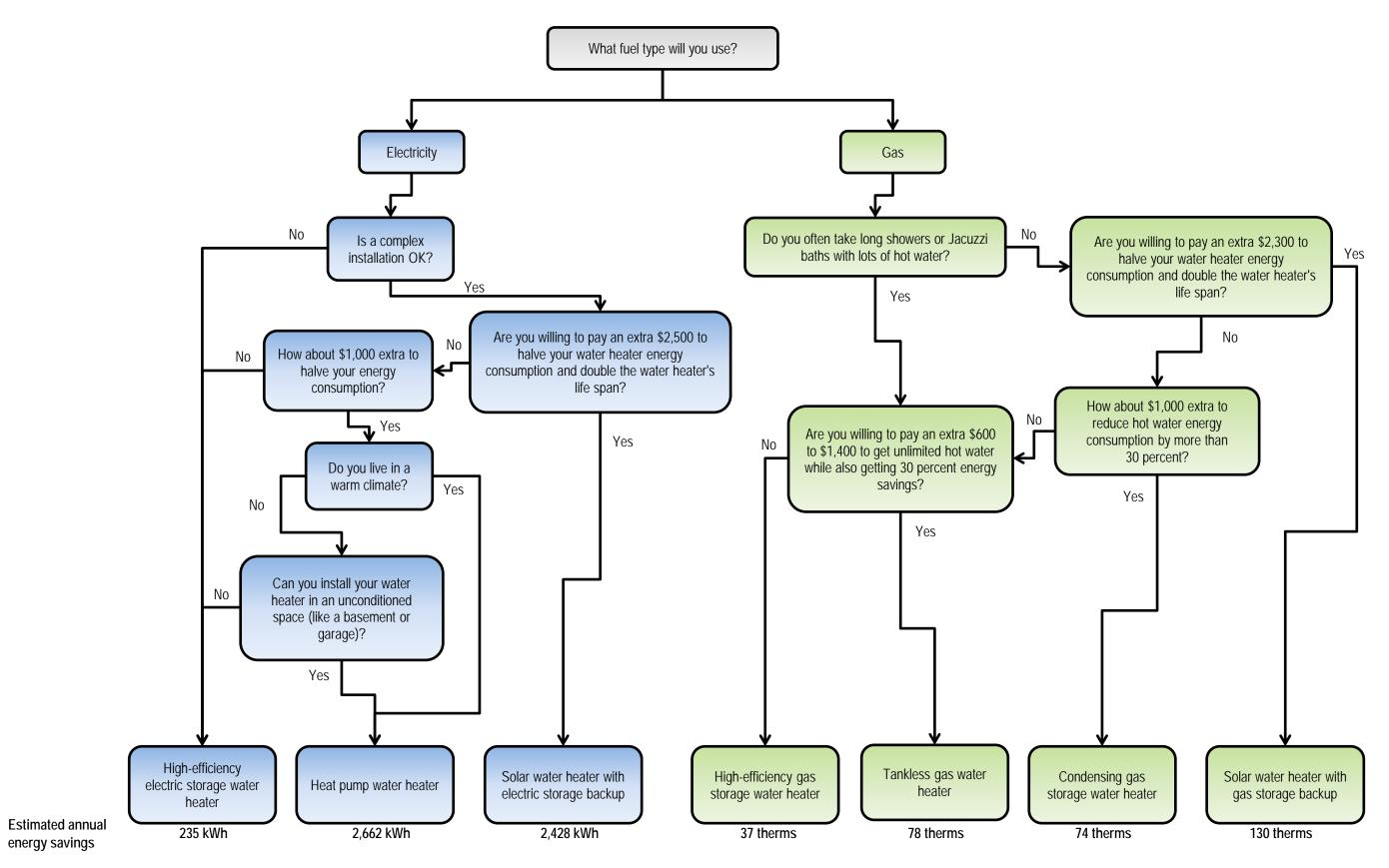
Notes: kWh = kilowatt-hour. Cost estimates referenced are representative of available 50-gallon (or equivalent) water heaters. Utility incentives may adjust relative incremental costs. Estimated annual energy savings are relative to a storage water heater at minimum federal efficiency standards.
