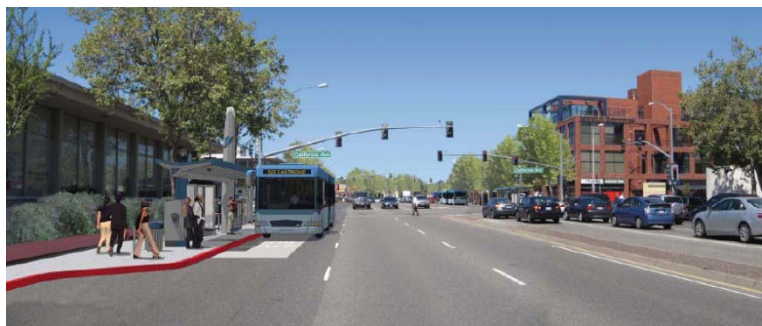
In Palo Alto, El Camino Real BRT will not include center-running transit lanes, but instead utilize widened sidewalks at bus zones – or bus bulbs – to improve transit access, amenity space, and passenger comfort. In addition to the improvements at California Avenue (above), VTA is planning for bus bulbs at the Charleston/Arastradero intersection. (Source: VTA)
