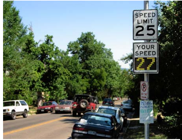
Speed feedback signs inform drivers of their speed and encourage them to drive at the posted speed limit.
