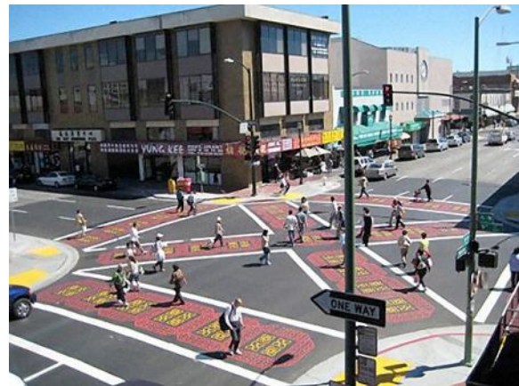
The City of Oakland installed a pedestrian scramble in its Chinatown, later adding pavement inlay designs to make crosswalks more visible.
