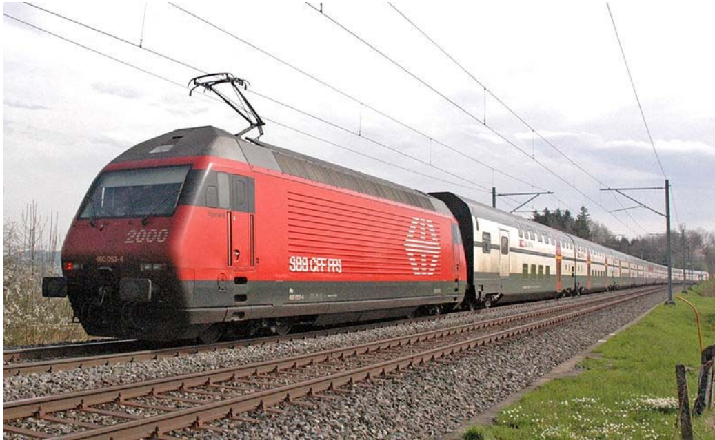
Well covered bogies by engine body of Swiss Engine type RE 460 (Lok 2000)
