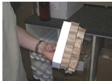
Cardboard packaging material is favored over polystyrene so it can be easily recycled
